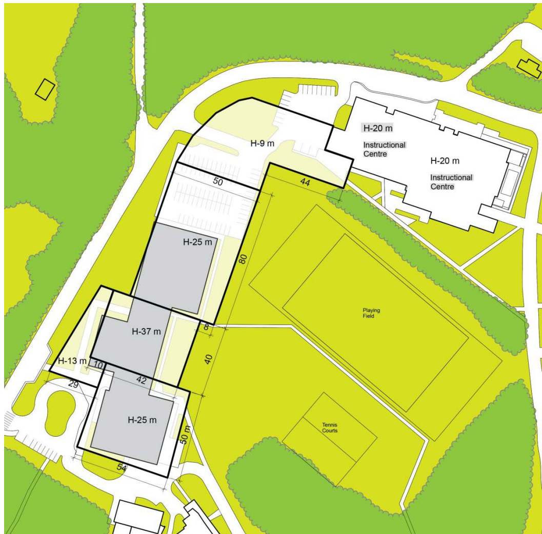
Plan showing all Phases Site 7, North Building Redevelopment, 2011 UTM Campus Master Plan Phase A envelope on the right stepping up to 5 storeys (6 storeys from Campus Green) from the existing Erindale Hall Residence (under construction); rising to 9 storeys in Phase B with a lower entrance court envelope; and dropping back down to 6 and 2 storeys in phase C at the left, to connect with the existing Instructional Centre. Existing Building, to be demolished, is shown in grey.
