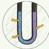
**2** U-shaped pipes are inserted into each borehole. Water is circulated through this system, taking excess heat from buildings in the summer and storing it underground for use in the winter.
