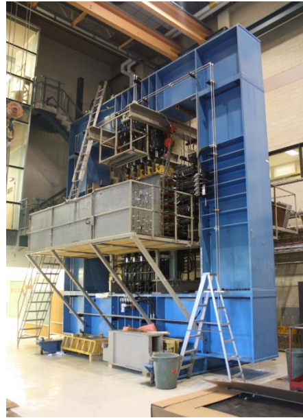
GB16 EXISTING EQUIPMENT (Left: Baldwin 1.2Mlbf hydraulic press; Right: Shell Element Tester)
