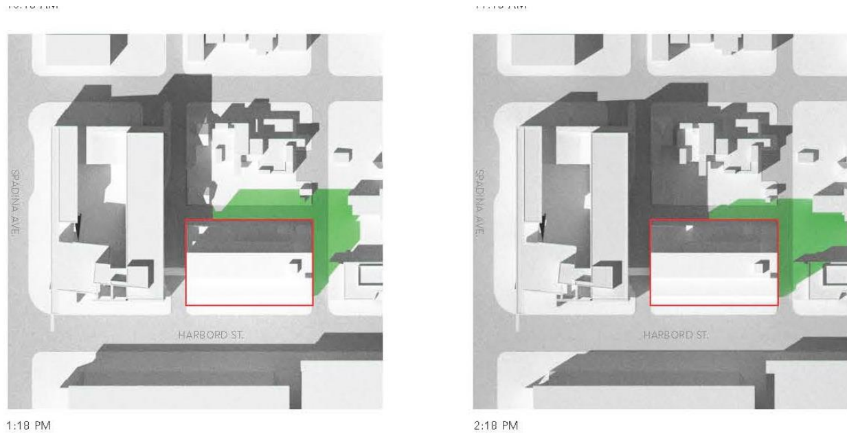
Figure 17 - Shadow Study Showing Graduate House and Harbord Residence on September 21: Image Courtesy of Michael Maltzan Architects / architects Alliance
