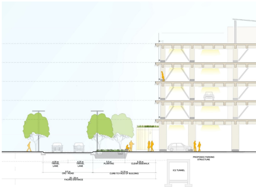
Building Section Showing relationship to new Campus Road at South Façade (Image by gh3*/ Behnisch Architekten)
