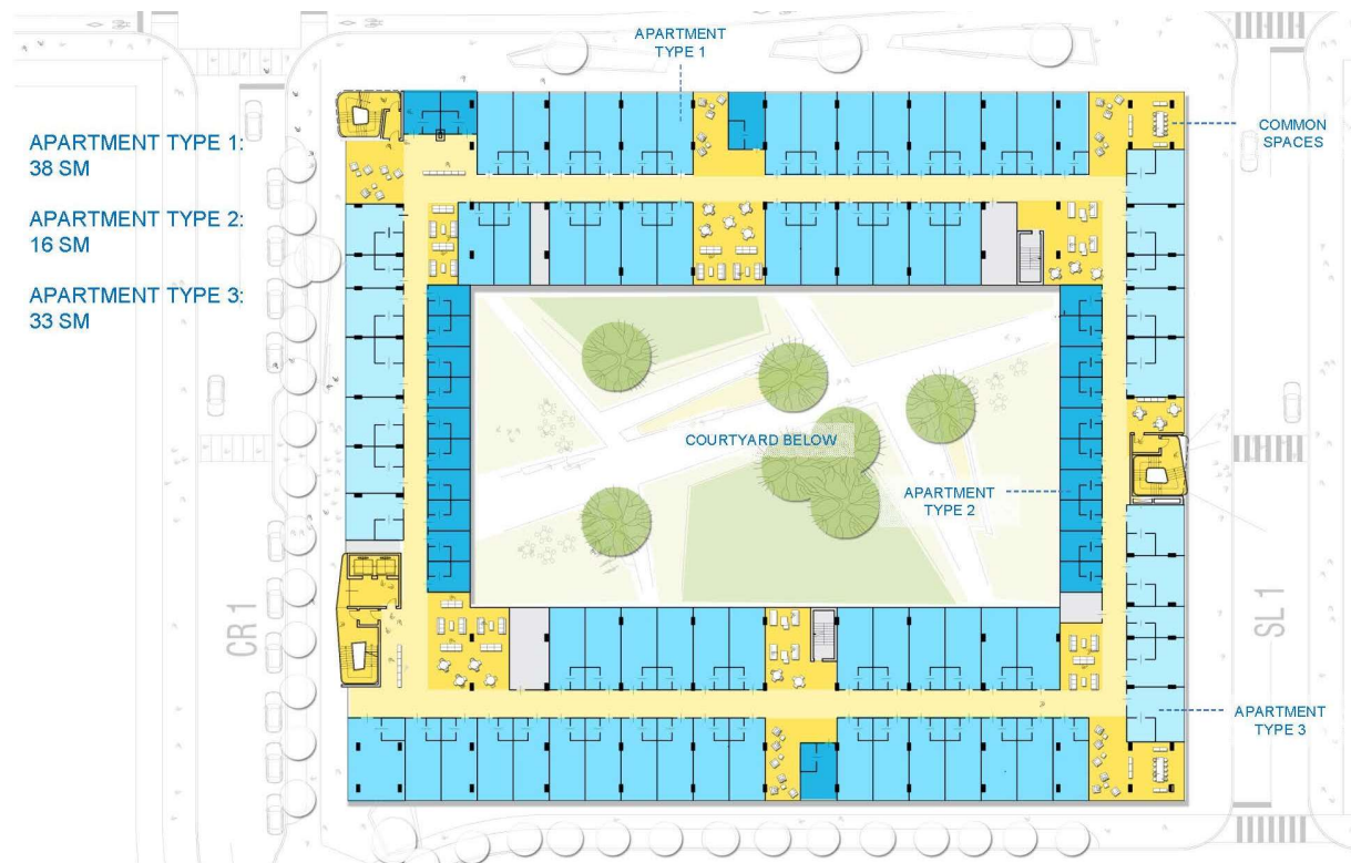
Plan Study showing potential future conversion to Student Residence through removal of central ramping (Image by gh3 + / Behnisch Architekten)
