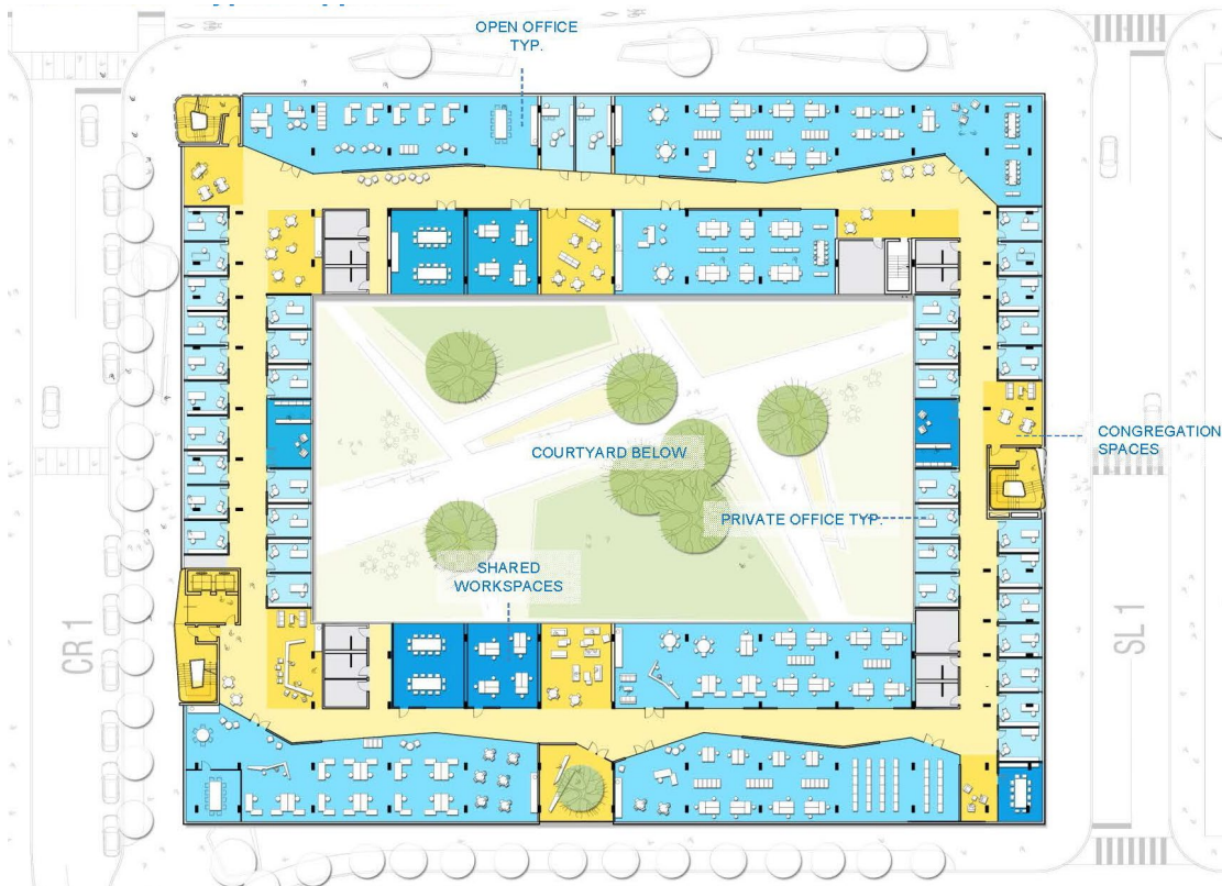
Plan Study showing potential future conversion to Office Use through removal of central ramping (Image by gh3 + / Behnisch Architekten)
