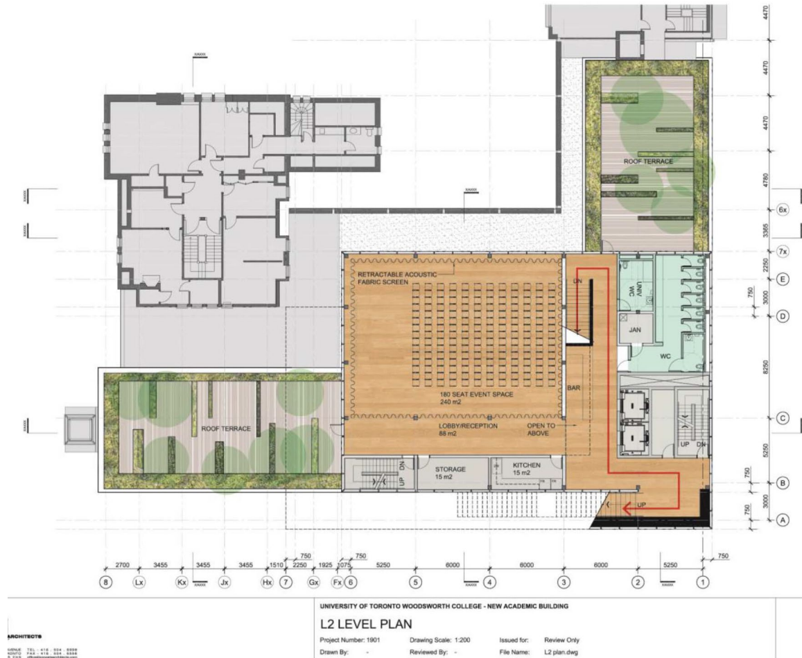
Event Floor Plan showing Accessible Green Roofs (controlled access) by Kongats Architects
