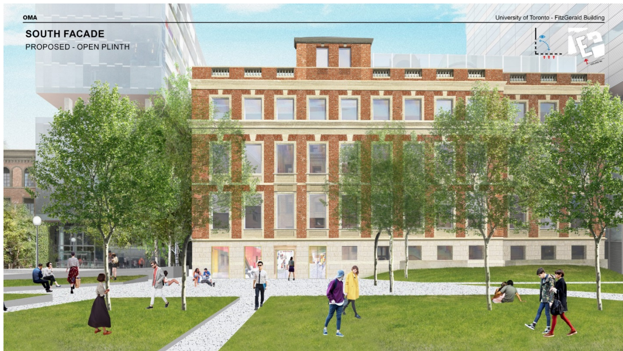
FitzGerald, showing the proposed South Façade off College Street. Note: the windows shown in the rendering propose single pane, triple glazing. An alternative approach may include metal screens to introduce divisions into the windows.
