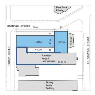
A tower is proposed at the eastern edge of the site. The tower is situated such that it minimizes shadowing to the green space immediately north along Harbord Street, while providing a structure of landmark significance at this important location on campus. The existing single level lecture theatre pavilion located at the intersection of St. George and Harbord Streets could be demolished to accomplish this envelope, or maintained as a podium.
