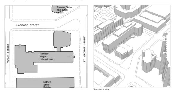
A 7-storey development envelope allows for the continuation of existing program matching the existing Ramsay Wright Laboratories building in height and floor level. The envelope extends north to bring the main address and building entry to the street, and provides an opportunity to enliven the streetscape with programming at ground level. The envelope anticipates an atrium/winter garden connection between the new structure and the existing Ramsay Wright building.
