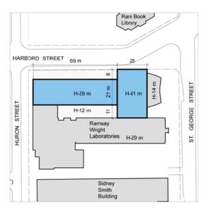
A tower is proposed at the eastern edge of the site. The tower is situated such that it minimizes shadowing to the green space immediately north along Harbord Street, while providing a structure of landmark significance at this important location on campus. The existing single level lecture theatre pavilion located at the intersection of St. George and Harbord Streets could be demolished to accomplish this envelope, or maintained as a podium.
