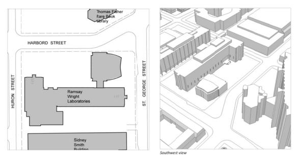
A 7-storey development envelope allows for the continuation of existing program matching the existing Ramsay Wright Laboratories building in height and floor level. The envelope extends north to bring the main address and building entry to the street, and provides an opportunity to enliven the streetscape with programming at ground level. The envelope anticipates an atrium/winter garden connection between the new structure and the existing Ramsay Wright building.
