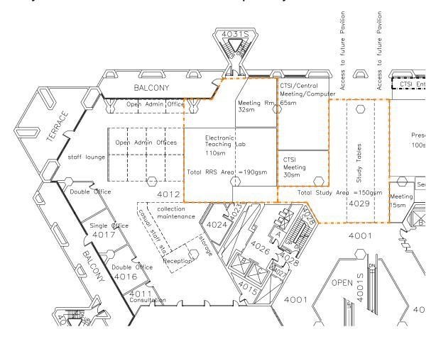
Note: Area outlined in orange indicates estimated area of new construction to be completed. The total study area is approximately 150sm and the total electronic teaching lab and meeting room area is approximately 190sm for a total of 340sm of new construction space.
